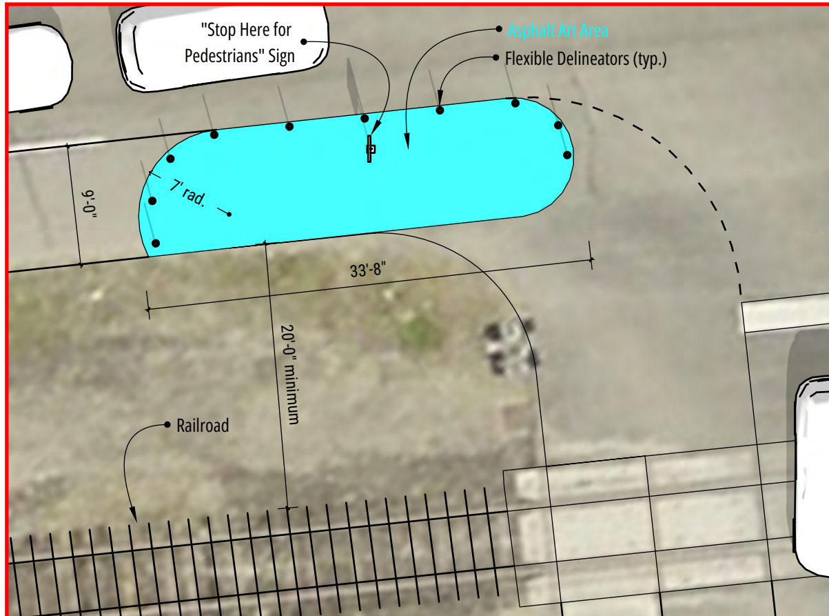
01 Enlarged Plan Southwest Corner | Art Shape Detail | Scale: 1"=10'-0"
